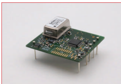
▲ Fig. 5 Syrlinks timing module with GNSS synchronization.
