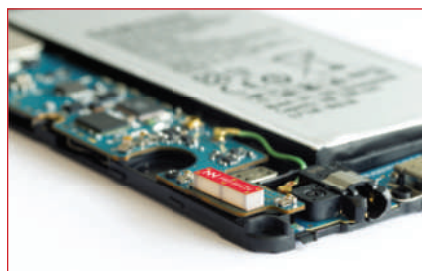
▲ Fig. 1 Antenna booster, measuring 12 mm × 3 mm × 2.4 mm, mounted on a corner of a smartphone PCB.
